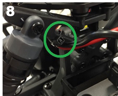
8 Connect the motor wires. Note the color sequence for proper polarity. Connect black to black and red to red. Reattach the wires with a zip tie.
