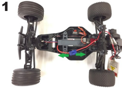
1 Disconnect and remove the battery.
