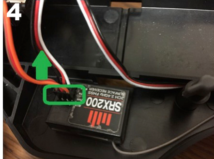
4 Pulling gently straight out, disconnect the ESC from the receiver (receiver is marked THR).
