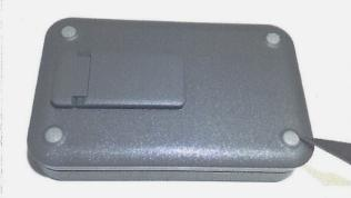
1. Carefully lift up the four rubber feet's and remove the four Philips screws
