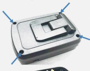
1. Remove the four Philips screws
